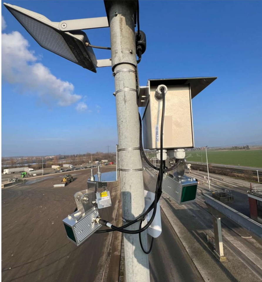
Fig.2: OWL EYE LiDAR sensors mounted on light pole to monitor stockpiles. © Sachtleben Technology GmbH.
