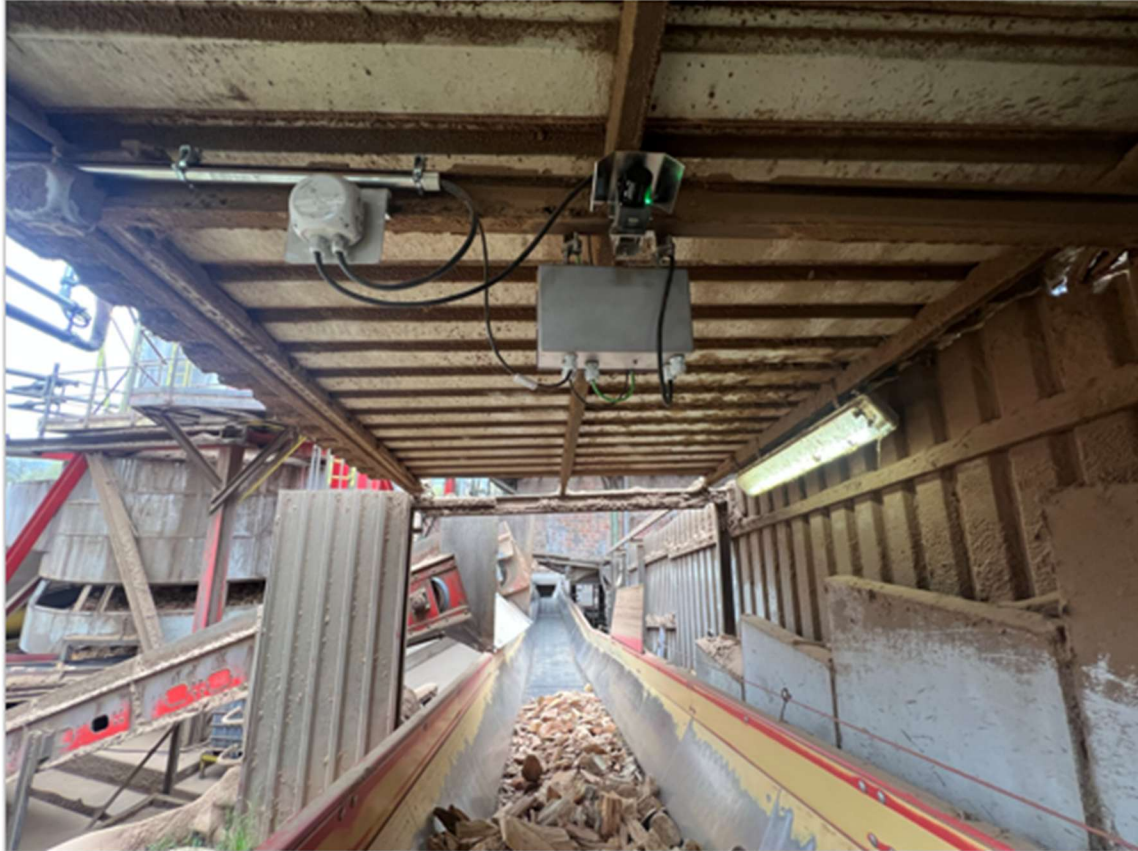
Fig. 4: OWL EYE LiDAR sensor above a conveyor belt continuously scans the cross-sectional profile of the material and provides detailed condition monitoring of the conveyor belt. © Sachtleben Technology GmbH.
