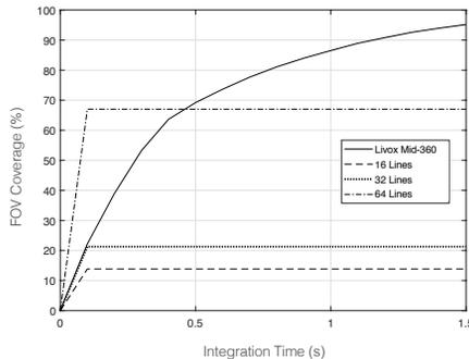
The FOV coverage of Livox Mid-360 and non-Livox LiDAR sensors using common mechanical scanning methods.
